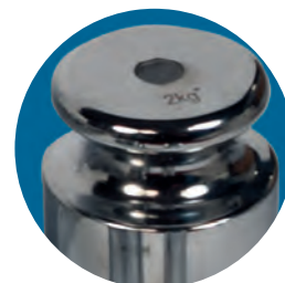
Top adjustment cavity
